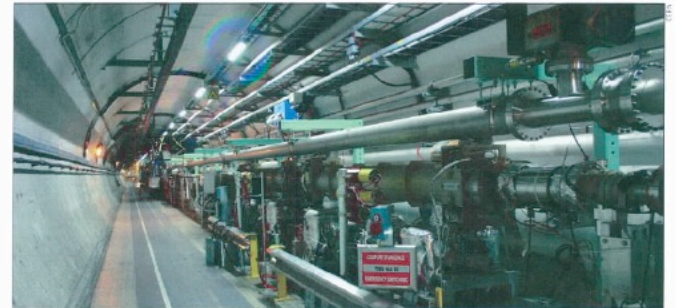
Loneley journey: A proton can travel more than 100 billion kilometers through the LHC's beam pipes without encountering a single residual gas molecule.
